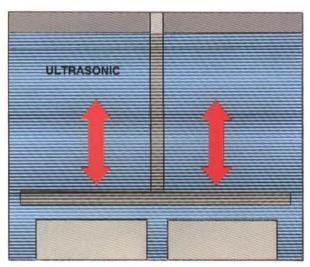
Ultrasonic cleaning is improved by using the oscillating platform to gently move the load throughout the ultrasonic working zone. Furthermore, ultrasonic stages can be alternated with turbulating stages. This is a particularly effective way to handle stubborn contaminants such as buffing or lapping compounds.
