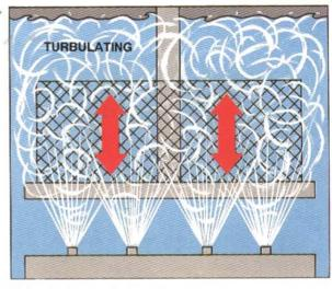
Combining platform oscillation with turbulent immersion washing / rinsing results in constantly changing flow patterns to provide an even flow of turbulance over, under, around and through components.
