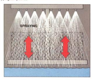
Combining platform oscillation with pressure spray washing / rinsing results in constantly changing spray patterns to minimize sheilding and improve coverage onto all surfaces of the parts.
