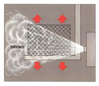
Using high volume hot air combined with changing air flow patterns created by the oscillating elevator provides rapid drying without excessive heating.
