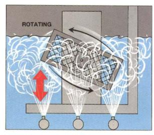
Using a Parts Rotator on an oscillating platform increases solution flow-breaking in and out of solution filling and draining blind holes - with each oscillation.
